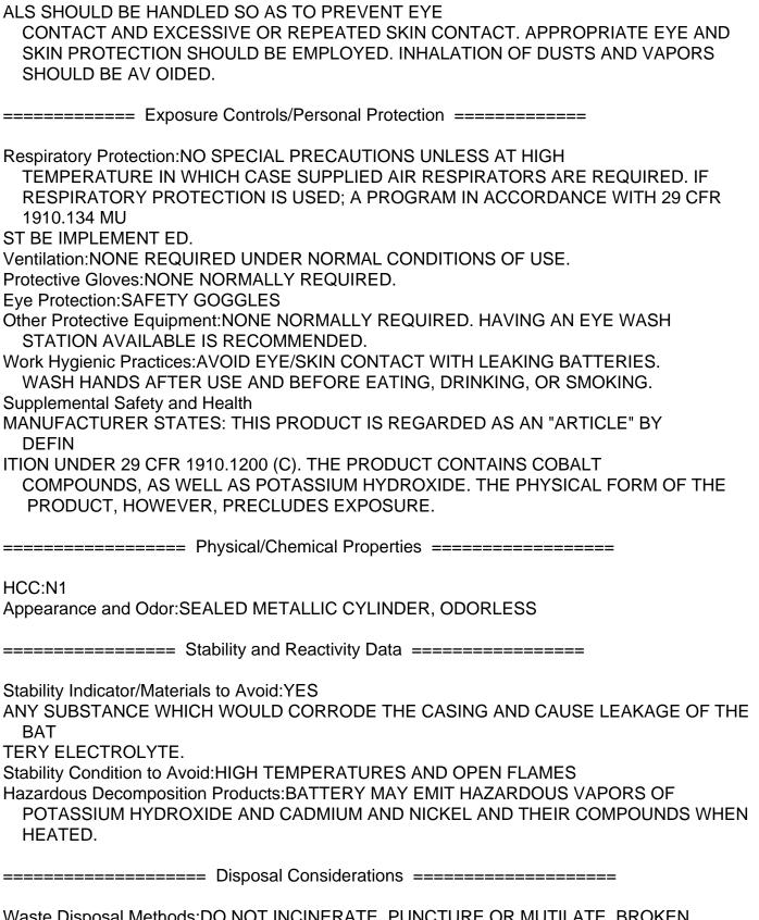
Waste Disposal Methods:DO NOT INCINERATE, PUNCTURE OR MUTILATE. BROKEN BATTERIES OR BATTERIES WITH LEAKING ELECTROLYTE CONSTITUTE HAZARDOUS WASTE. CONSULT WASTE DISPOSAL OFFICIALS FOR ADV
